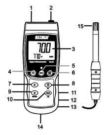
**Notes:** Items 11 – 13 are located behind the snap-off compartment cover on meter's right side. Battery compartment, tilt stand, and tripod mount are located on the rear of the instrument
