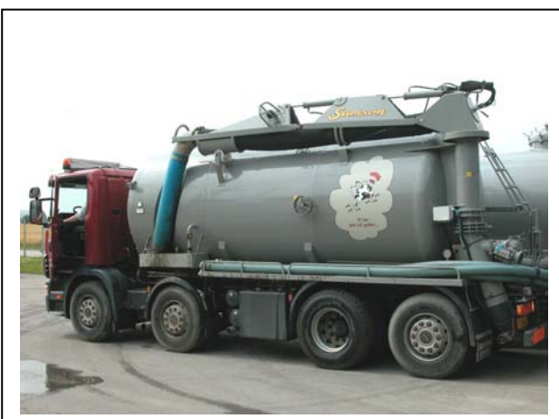
Road tanker for transportation of animal manure in Denmark
