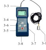
3-1 Accelerometer3-2 Display3-3 Input Connector3-4 Hold key
